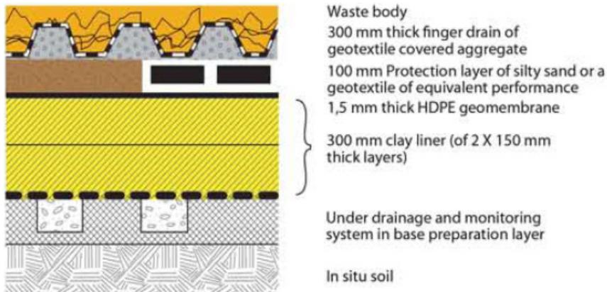
**Figure 10.4:** Class C Liner System
